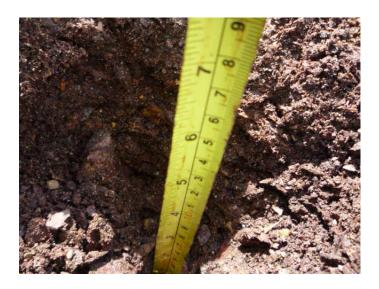
Trip zones found at edge of surface. Recommend build up ground levels to remove trip hazard (see above) - Low to Medium risk.
