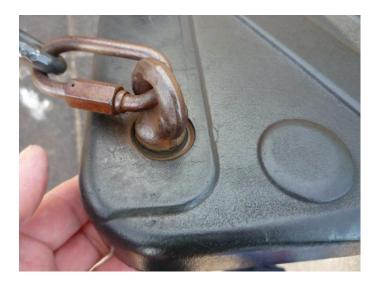
Recommend to remove shackle bolt and check bush and shackle pin wear, replacing if necessary.
